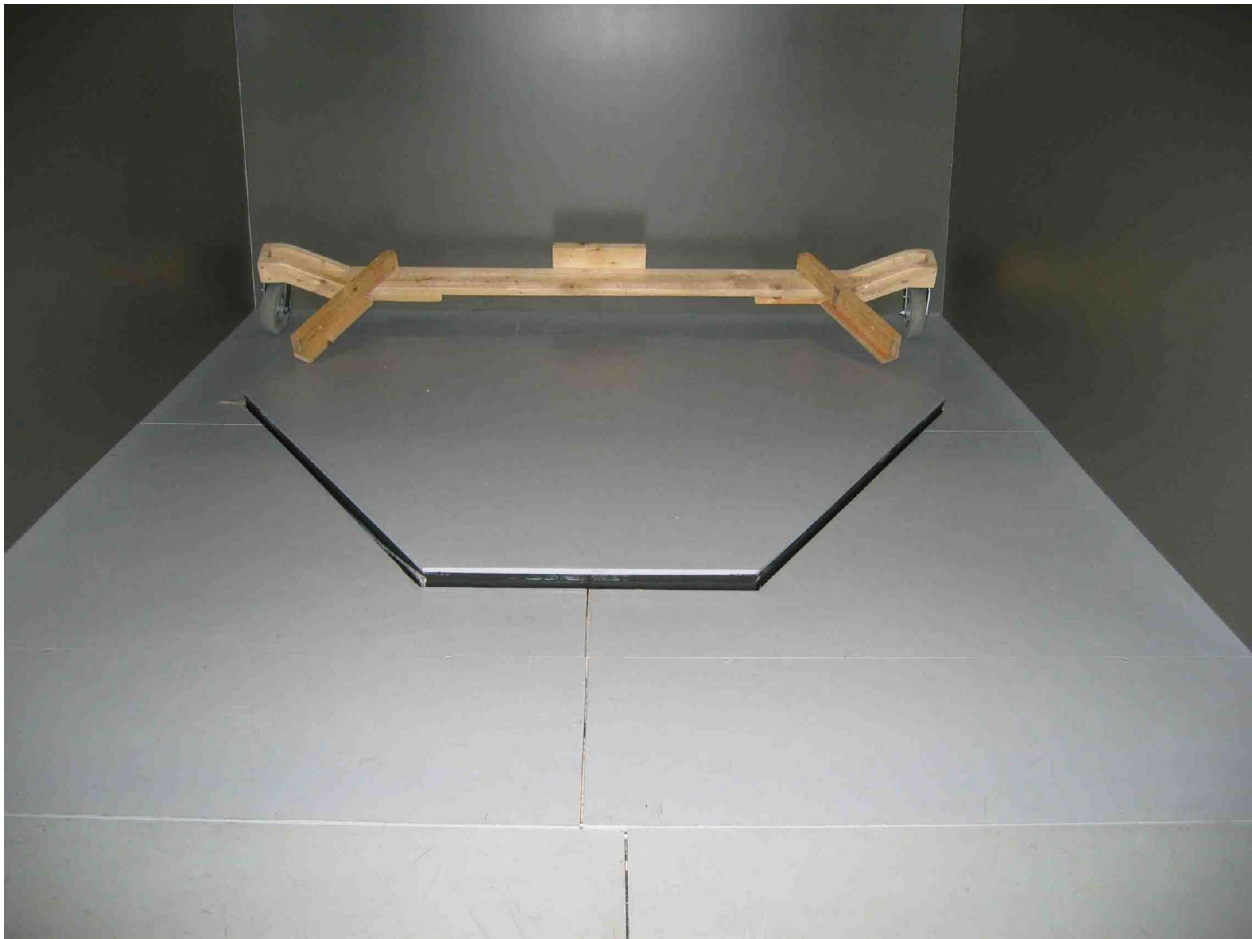
Figure 7. Placement of the long beam used to hold the motion platform cover.
