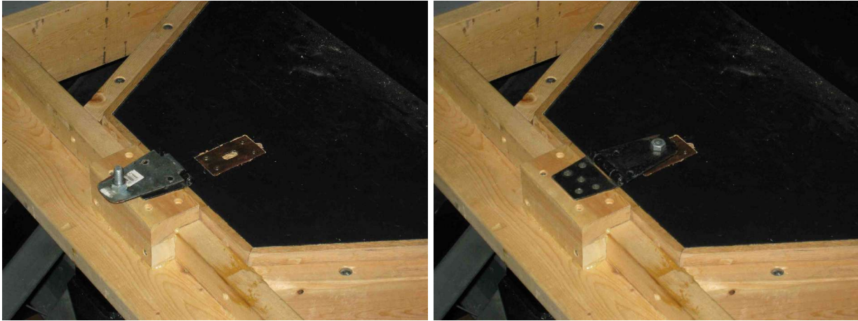
Figure 16. (a) MOOG chair carrier unlatched from chair. (b) MOOG chair carrier latched to chair.
