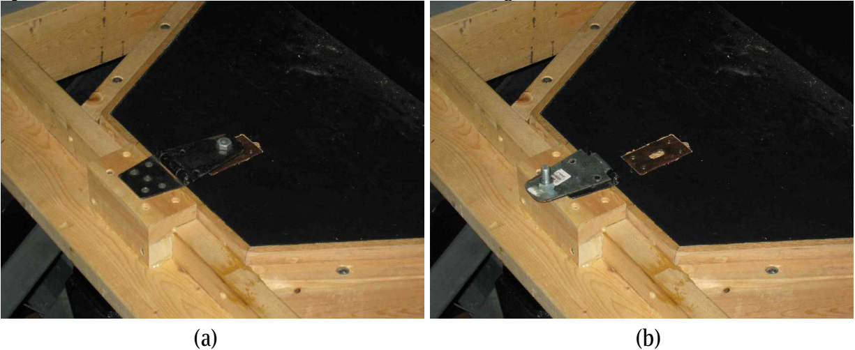
Figure 11. (a) MOOG chair carrier latched to chair. (b) MOOG chair carrier unlatched from chair.
