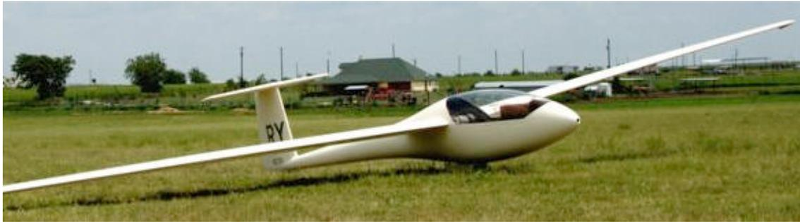
15 Meter with flaps and trailing edge spoilers/dive brakes, Parallelogram stick, Heel brakes, Integrated ballast tanks (115 liters) Competition sealed, Tost CG and nose releases, In-flight adjustable rudders and seat back, Press-to-set trim. Panel: ASI, Compensated 1.2 sec Variometer with audio, Compensated 1.7 sec Variometer with 9v backup power source, Altimeter, Averager, Speed-to-fly calculator, Compass, Oxygen regulator, Voltmeter, 720 Channel transceiver w/Boom mike
